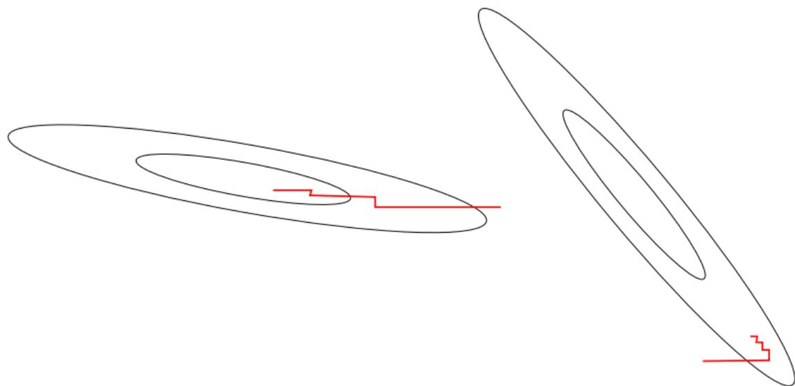
Left figure is better. It can tolerate a higher delay parameter  $\tau$  and thus more cores working asynchronously.
